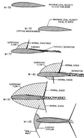
Figure 2.9. Transonic Flow Patterns (Sheet 1 of 3)
